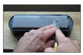
Woodcarvers use the benchstone to work on the *outside* bevel of the carving gouge, which must be sharpened to the correct angle (15-20°).
