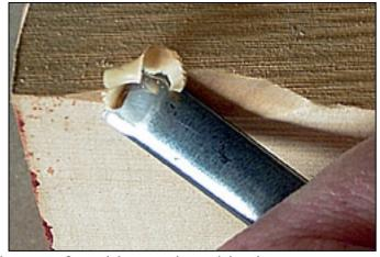
With an inside bevel, a gouge can be comfortably used upside down, losing that tendency to jig and dig in that a flat face to the tool gives. The versatility of the tool is thus greatly increased with a carver matching the profile of the gouge to the roundness of the wood surface when shaping convex surfaces.
