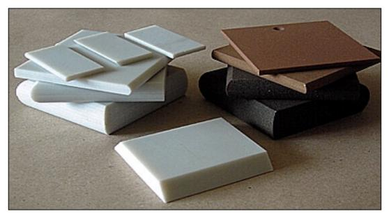
To the left, the fine Arkansas stones; these take on a translucent quality with honing oil. To the right, the matching coarser stones: the thicker slipstones are a coarse grit; the thinner slipstones are a medium grit, there being less metal to remove.
