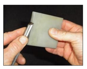
gouge as closely as possible then (with oil) rubs the stone back and forth in cannel at a tight angle (5-10°), inspecting the metal surface continually to monitor the abrasion.
