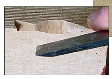
In contrast to carpentry chisels, gouges are principally used with the main, outer bevel to
