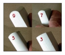
**Note:** Because there is a huge number or sweeps (the radii of the arc of the gouge edge) and widths, it is impossible for these slipstones to fit all of them perfectly. However, where they don't they should fit a lot closer than with previously available slipstones. Also, for the cost of the slipstone, the carver gets 4 profiles, rather than one.
