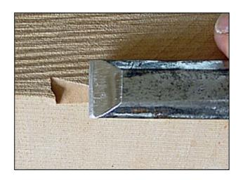
The chisel cannot exit the cut back to the surface without 'chattering' because there is nothing for the cutting edge to pivot on.
