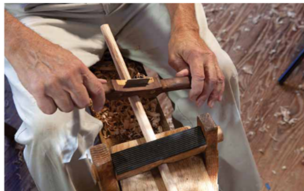
Larry Barrett's round rung scraper. The blade is from an old saw blade with a 3/4"-diameter half-circle at the cutting edge. Shifting it just a little bit one way or the other gets at half the circumference of the rung without repositioning the rung.
