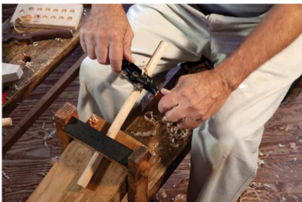
Shaving the rungs is much like what you did on the posts. Same idea, different scale.
