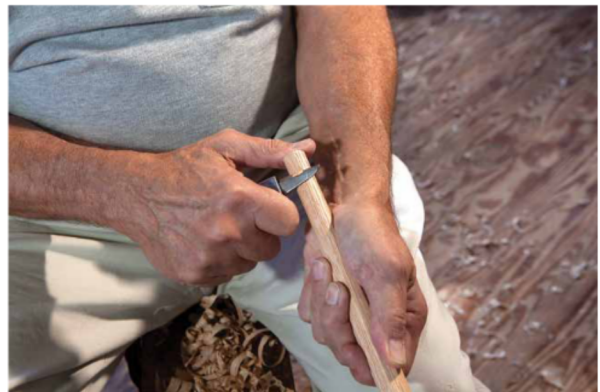
Slicing off the radial side of the tenon. Keep your thumb back out of the way as you pull the knife upward.
