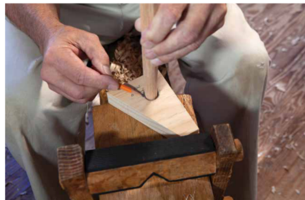
Marking tenon length in a test hole.
