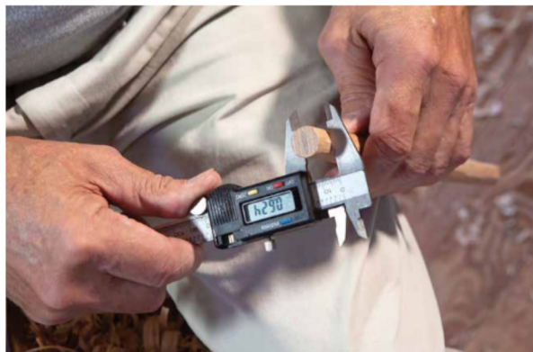
Measuring the tenon diameter with the digital calipers. The flats on the radial sides of the tenon are undersized to reduce the chance of splitting the post.
