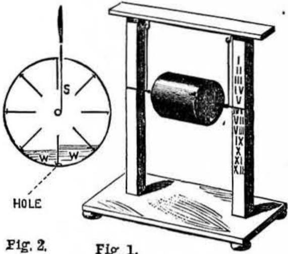
Fig. 1.—Water Clock Diagram. Fig. 2.—Section of Cylinder, showing Divisions and small Holes in each; also the Water and String (W S).
