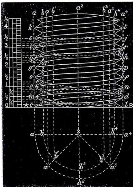
Fig. 15.—Double-Thread V-Screw ( $1\frac{1}{2}$  in. diam.).
