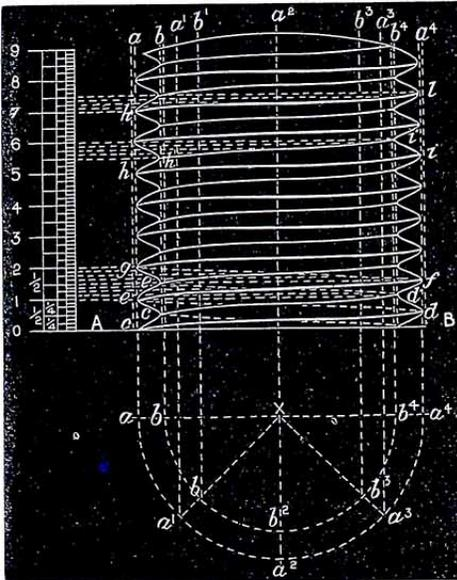
Fig. 14.—Single-Thread V-Screw ( $1\frac{1}{2}$  in. diam.).
