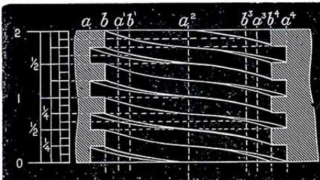
Fig. 18.—Nut for Double Square Thread Screw.
