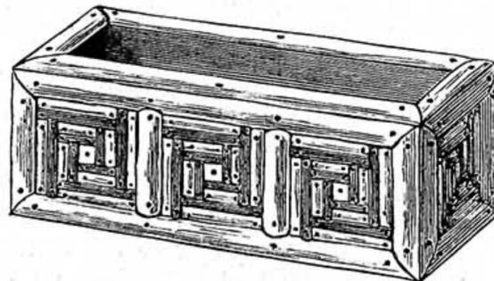
Fig. 4.—Window Box made from Raisin Box.
