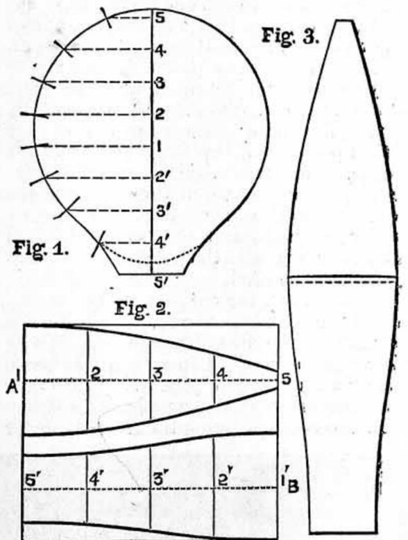
Fig. 1.—Pattern or Model for Toy Balloon. Fig. 2.—Gore set out in Two Parts on Tissue Paper. Fig. 3.—Parts cut out and joined to form Gore.
