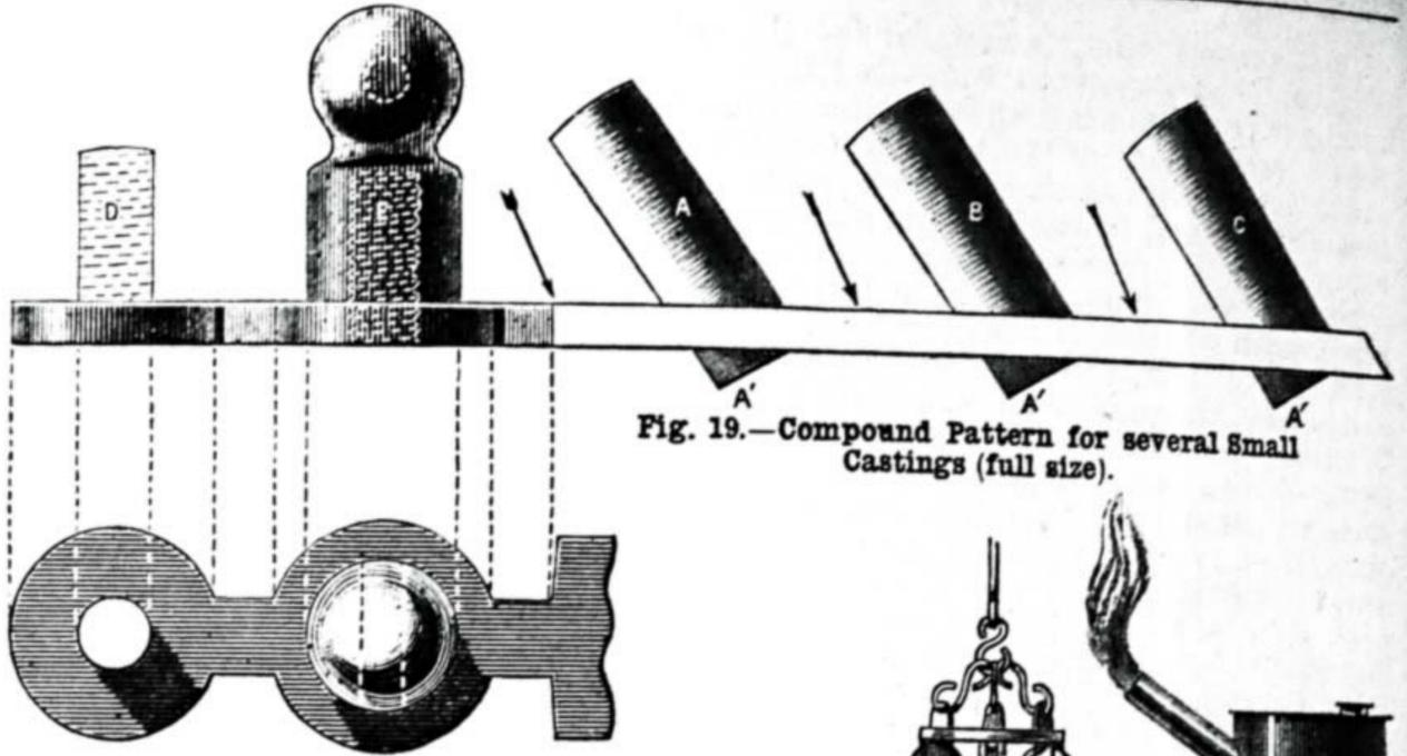
Fig. 19.—Compound Pattern for several Small Castings (full size).
