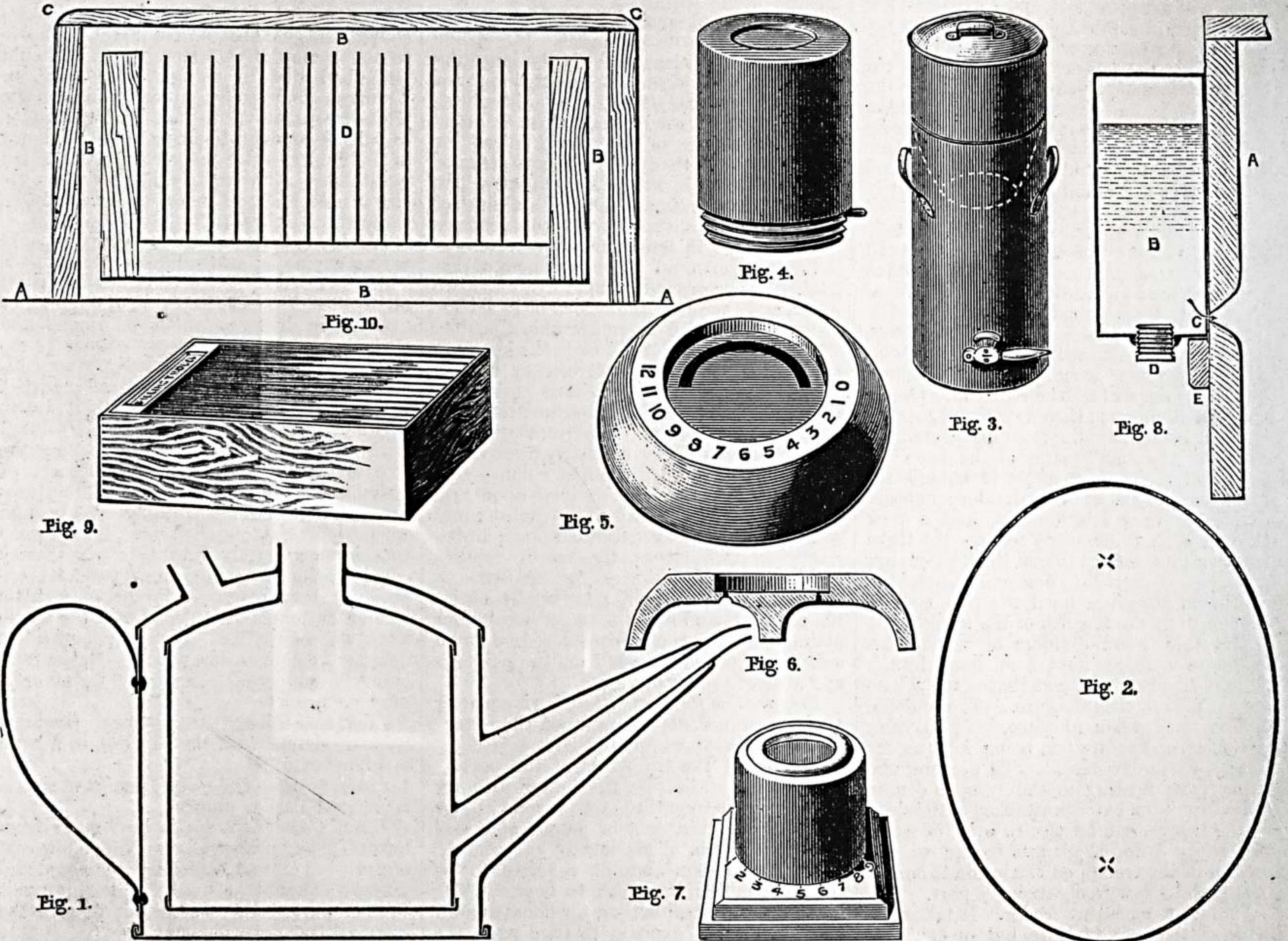
Fig. 1.—Section of Wax Smelter. Fig. 2.—Pattern of Bottom. Fig. 3.—Honey Ripener and Strainer. Fig. 4.—The Raynor Feeder: Feeding Bottle. Fig. 5.—Ditto, Stand. Fig. 6.—Ditto, Section of Stand. Fig. 7.—Square Base Feeder. Fig. 8.—Section of Hone's Dummy Feeder—A, Dummy; B, Syrup; C, Holes; D, Screw Cap; E, Slip to sustain Tin. Fig. 9.—General View of Rapid Feeder. Fig. 10.—Cross Section of Ditto—A A, Level of Top of Frames; B, Bee Space; C C, Top; D, Trough.
