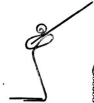
Fig. 14.—Clip for holding Cap.
