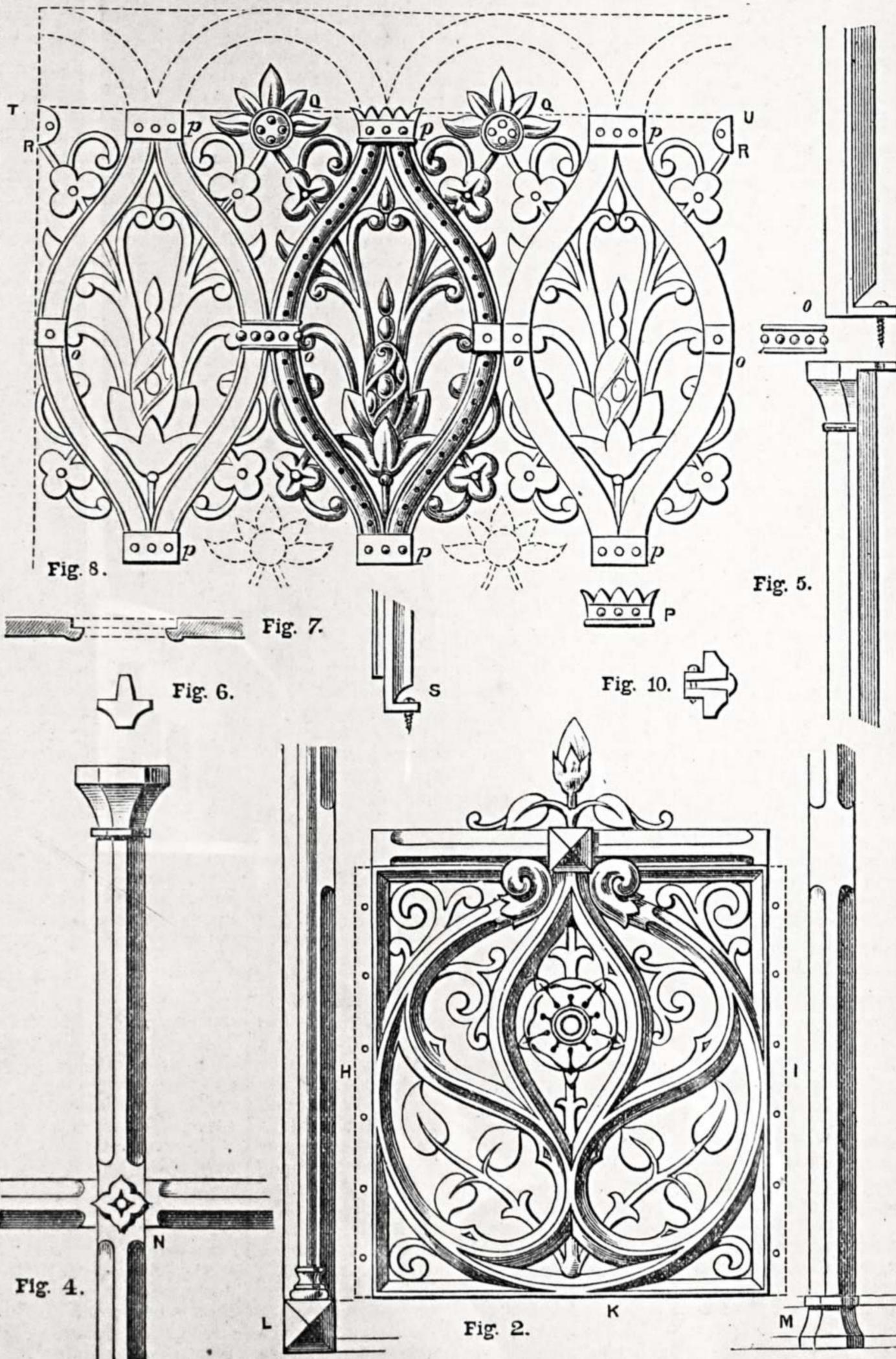
Fig. 2.—Panel for Bottom of Window. Fig. 4.—Mullion and Transom. Fig. 5.—Attachment of Head Panel to Mullion. Fig. 6.—Section of Glazing Bar. Fig. 7.—Rebate for Coloured Disc. Fig. 8.—Ornamental Window Panel. Fig. 10.—Section showing Mode of Joining Square Forms.
