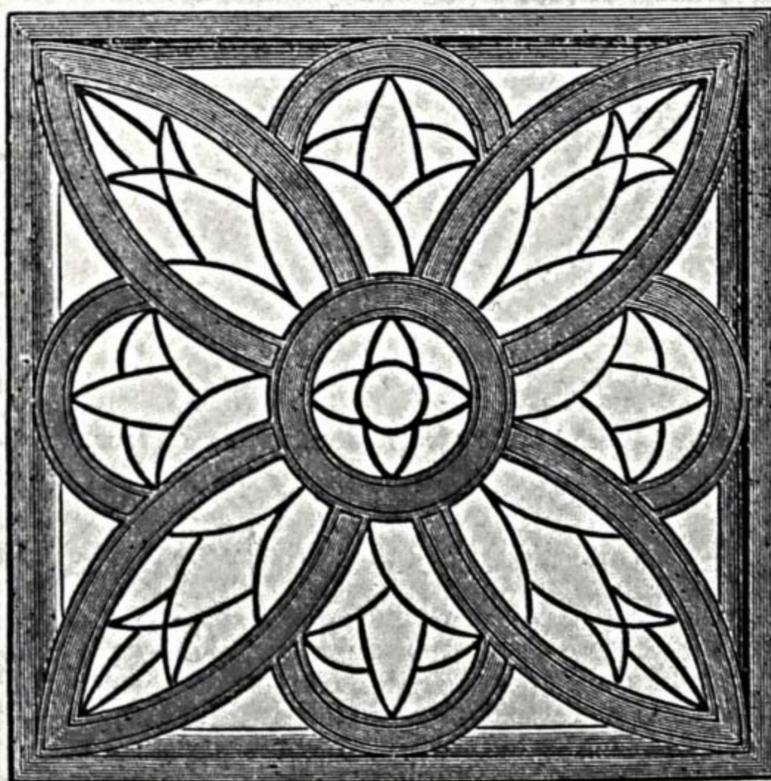
Fig. 9.—Iron Frame with Lead Glazing.
