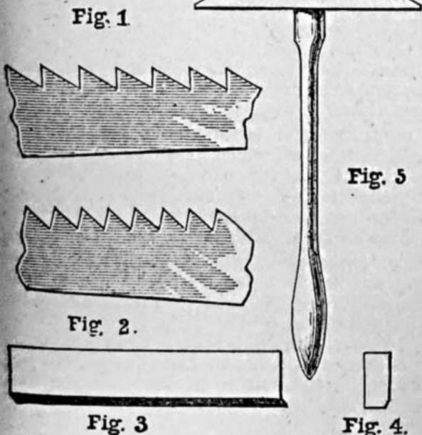
Fig. 1.—Ripping Teeth. Fig. 2.—Cross-Cutting Teeth. Fig. 3.—Setting Anvil. Fig. 4.—Steel Bevel. Fig. 5.—Setting Hammer.
