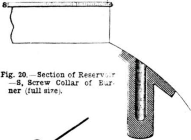
Fig. 20.—Section of Reservoir—S, Screw Collar of Burner (full size).
