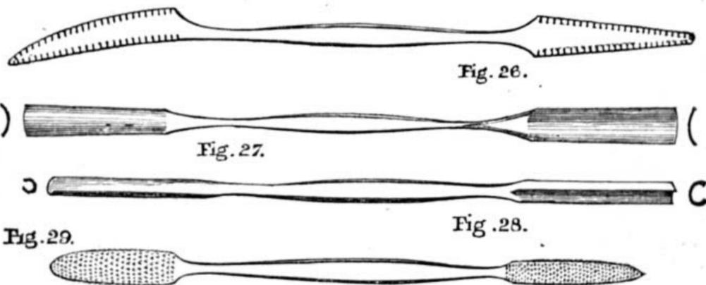
Fig. 26.—Saw-set Plaster Scraper. Figs. 27, 28.—Plaster Gouges. Fig. 29.—Plaster Ruffle.
