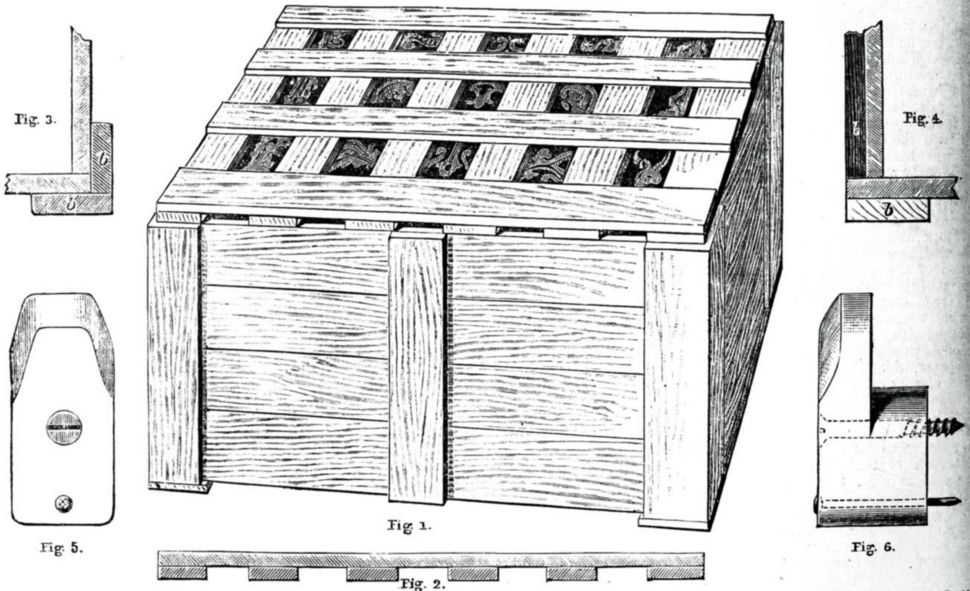
Fig. 1.—Perspective View of Packing Case with Open Lattice Lid, showing Carved Work inside. Fig. 2.—Longitudinal Section of Lid. Fig. 3.—Section through Corner, showing Overlapping of Battens *b, b*. Fig. 4.—Section through Backboard, showing Battens on End and below Backboard. Figs. 5, 6.—Plan and Side View of Batten for fixing Articles to Backboard when screwing would spoil them.
