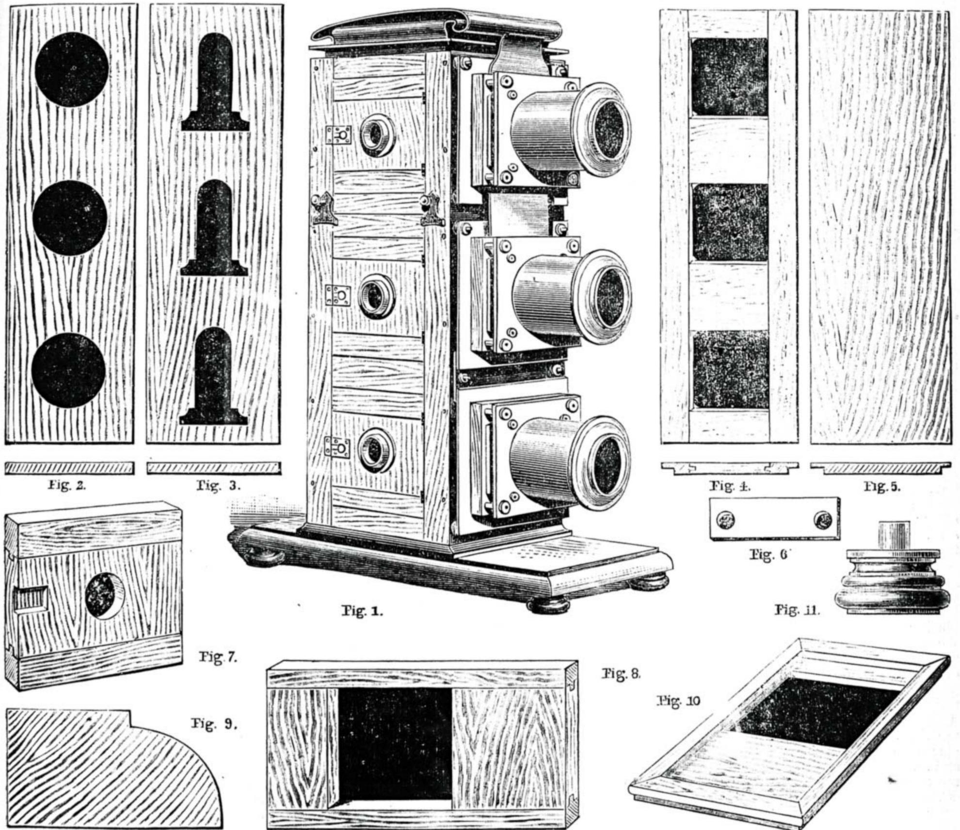
Fig. 1.—Triunial Lantern complete. Figs. 2, 3, 4, 5.—Plans and Sections of Front, Back, and Side of Lantern Body. Fig. 6.—Brass Angle Plate for Door Openings. Fig. 7.—Plan of Door. Fig. 8.—Plan of Baseboard. Fig. 9.—Moulded Bead for Baseboard. Fig. 10.—Baseboard complete, showing Under Side. Fig. 11.—Turned Foot for Baseboard.
