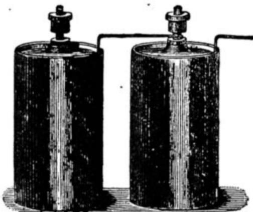
Fig. 1.—Gassner Dry Battery: Round Cell.
