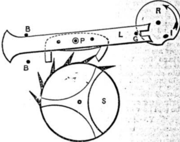
Table Roller Lever Escapement—L, Lever; P, Pallets; B, Banking Pins; G, Guard Pin; I, Impulse Pin; R, Roller; S, 'Scape Wheel.
