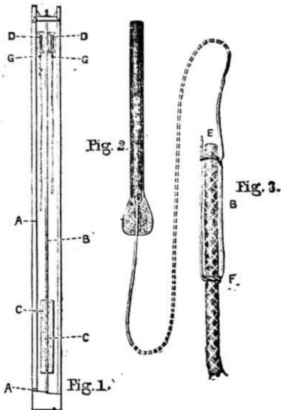
Sash-Hanging Parts. Fig. 1.—Sash Beadings, etc. Fig. 2.—Lead flattened and then bent round Cord. Fig. 3.—Method of fastening Mouse on to End of Sash Line.
