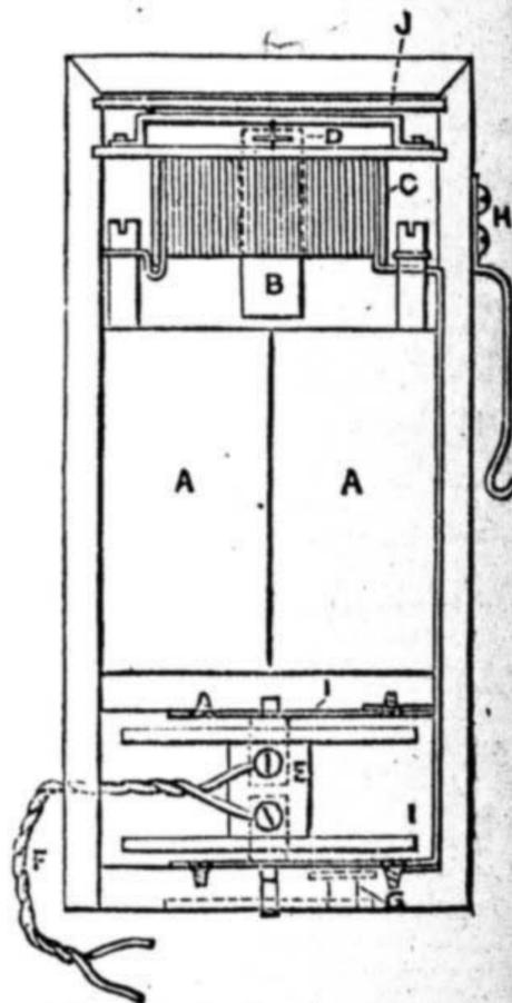
Improved Electric Testing Apparatus—A, Battery; B, Magnet; C, Coils; D, Needle; E, Spool; F, Testing Cords; G, Winder; H, Suspending Hook; I, Contacts; J, Glass Cover.
