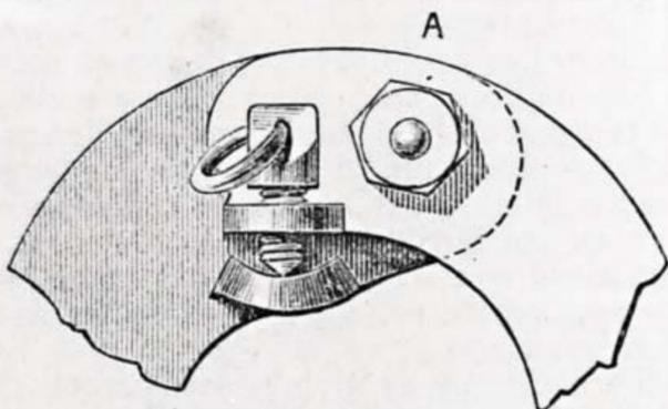
Fig. 1.—Joint of Metal Tree with Joint-Pin and Nut (A).
