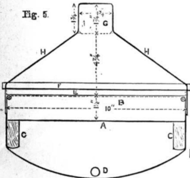
Fig. 4.—Wire Netting and Frame. Fig. 5.—Section through Extractor at Upper Strap. A, Netting; B, Space for Comb; C, Frame; D, Tube; E, Shutter; F, Cleat on Shutter; G, Handle; H, Strap.
