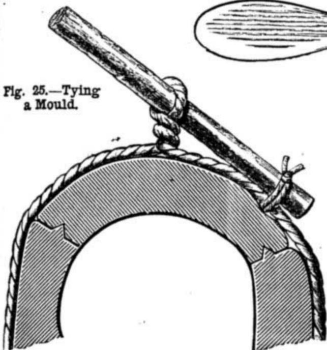
Fig. 25.—Tying a Mould.
