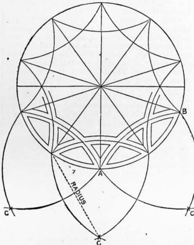
Fig. 16.—Setting Out of Double Pentagon in Fig. 6.
