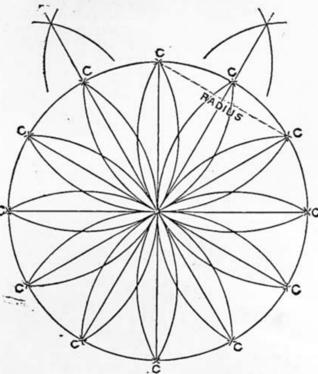
Fig. 14.—Setting Out of Double Hexagon in Fig. 9.
