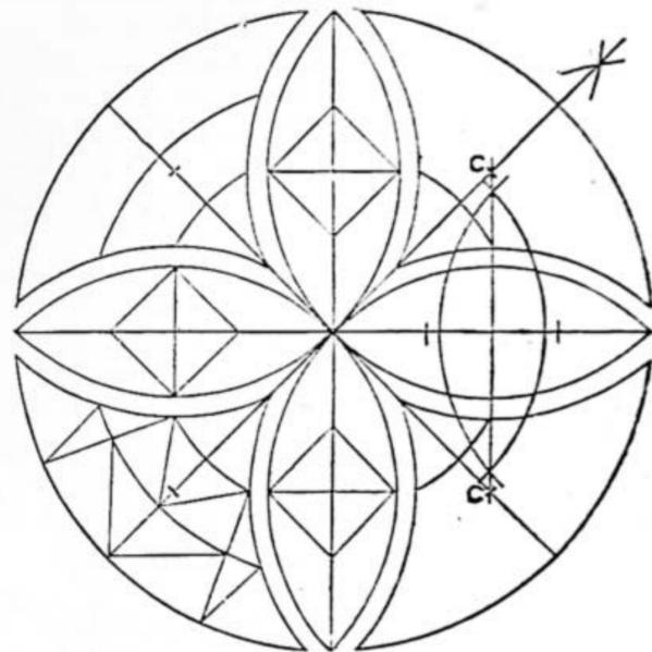
Fig. 15.—Setting Out of Quatrefoil in Fig. 6.
