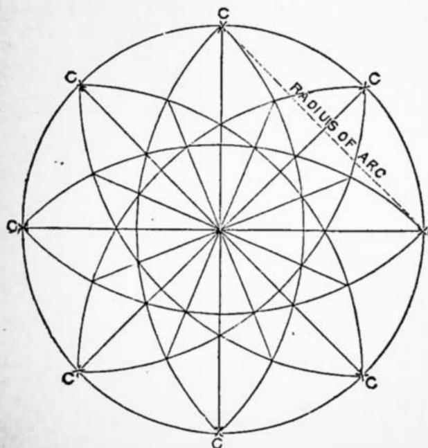
Fig. 13.—Setting Out of Octagon in Fig. 9.
