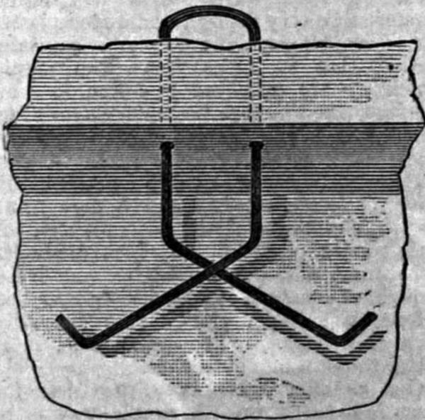
Fig. 18.—Wire Loop arranged in Mould.
