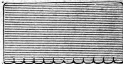
Fig. 19.—Plaster Drag (Scale, half size).
