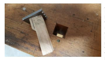
Joel's workbench is based on the Frank Klausz workbench in *The Workbench Book* by Scott Landis and has a traditional tail vise and square dog holes (in addition to round ones). The obvious method of setting up a planing stop on this type of bench is to just screw the stop onto a square block of wood and clamp it into the tail vise when needed. This took all of three minutes to do, and for that type of bench, it's a great solution.
