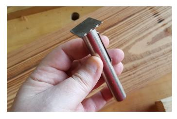
In the industrial age, there were a bunch of not-very-good manufactured stops. The Stanley #207 Bench Stop (1929-1974) was a small stop on top of a round shaft that could fit into a round hold in your bench. The Stanley #207 we have is very dull and doesn't dig deep enough (or at all actually). Also for reasons that don't make sense, it has a 9/16" shaft not a ¾" shaft.
